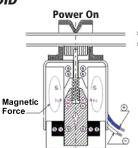
Current flows to the coil, the electromagnetic force is created in such direction that the attractive force increases and becomes stronger than the spring. Then, the plunger moves towards the pole piece.
