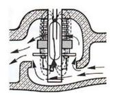
A magnet equipped shuttle is displaced at the proper calibrated flow of liquid to actuate the hermetically sealed reed switch. At flow rates under the set point, clearance is provided for the liquid to continue to flow. When flow rates exceed the
