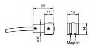
Magnet sensor for surface measurement
