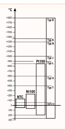
Selecting the right type of temperature sensor depends on your measuring task. For example, thermocouples, resistor-based sensors (Pt100 and Ntc) and pyrometers (infrared sensors) are available.
