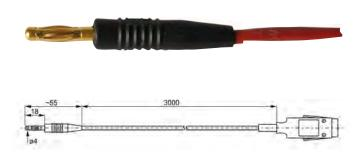
Measuring element PT100, 4-conductor class B, integrated in the socket of a 4 mm laboratory connector made of brass (goldplated). Plug-in laboratory sensor Order no. FPA414
