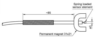
Magnet sensor For surface measurement
