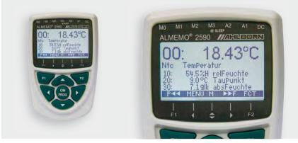
ALMEMO<sup>®</sup> professional measuring instrument with data logger function,
