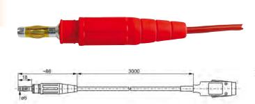
Measuring element PT100, 4-conductor class B, integrated in the socket of a 6 mm laboratory connector made of brass (ni-ckel-plated).
