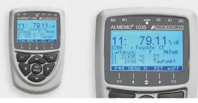
Reference measuring instrument for humidity High-precision measuring with Pt100 psychrometer Resolution Temperature 0.001 K Relative humidity 0.01 % Dew point 0.01 K
