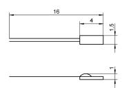
Meas. element: Pt100, Class B \* Measuring tip: Operative range -40...+400 °C Ceramic chip sensor Connection wires: 10 mm, bare Ceramic chip sensor **Order no. FP0802**
