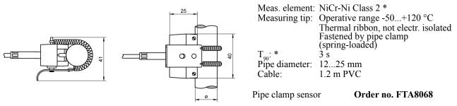
For surface measurement on pipes
