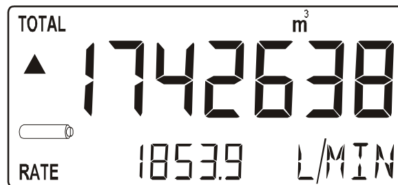
Fig. 4: Example of low-battery alarm
