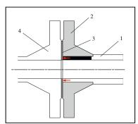
made of steel grade AISI 5LX / 1.1106. Flanges made of stainless steel AISI 321 / 1.4541 are optionally available.
