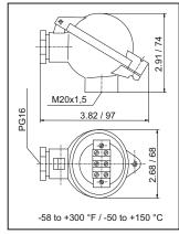
Plug connection **Terminal connector** housing
