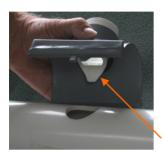
5. Place the top half of the saddle with the alignment slot inside the sensor housing on the downstream side, over the pipe so that the mount fits into the drilled hole.
