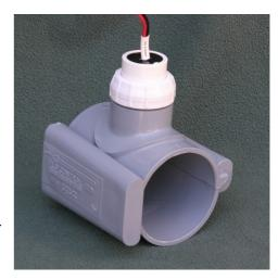
The flow sensor insert, held in place with a retaining nut, contains the detection circuitry and carries the unique four-bladed impeller on a transverse axle. The insert attaches to a housing that controls the location and alignment of the impeller. The housing is mounted in a PVC saddle therefore no additional mounting hardware is required. The axle and impeller along with the sealing o-ring are replaceable in the field.
