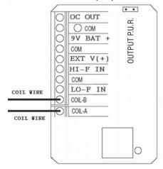
Connect either coil wire to COIL\_A terminal.
