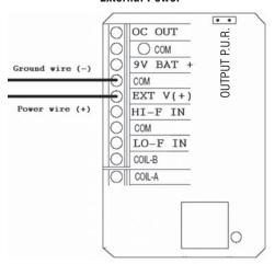
Connect power wire (7-30 VDC) to **EXT\_V(+)** terminal. Connect ground wire to any **COM** terminal.
