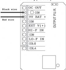
Connect battery (included) red wire (+) to **9V\_BAT+** terminal. Connect battery (included) black wire (-) to any **COM** terminal.
