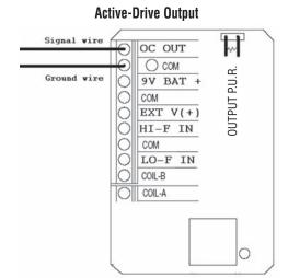
Connect signal wire to **OC\_OUT** terminal.
