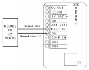
Connect signal wire to **HI-F\_IN** terminal. Connect ground wire to any **COM** terminal.
