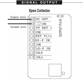
Connect signal wire to **OC\_OUT** terminal.
