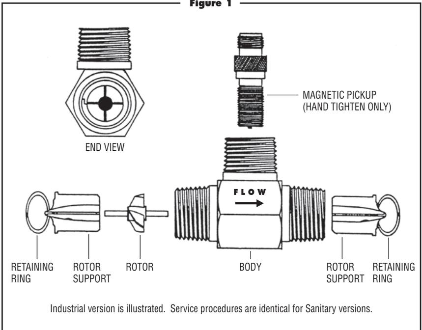
The turbine flowmeter should be installed in a location where the process line will remain full of liquid at all times. Otherwise, when the process line becomes empty and a valve is opened, the high velocity fluid hitting the turbine flowmeter rotor can cause severe damage.
