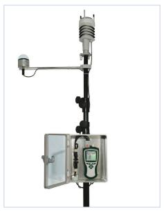
Universal mobile weather station for measuring a wide array of meteorological data, e.g. wind direction, wind velocity, relative atmospheric humidity, temperature, atmospheric pressure, rainfall quantity and intensity, and global radiation Quick and easy to install, robust design, and various power supply options (rechargeable battery, solar cell, car adapter)
