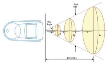
from 1km? Yes as long as the FOV is filled by the target. Also, many IRTs measure in the 8um to 15um wavelength band where the atmosphere is almost totally transparent.
