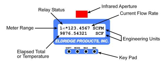
Meter Range — indicates the active meter calibration range (1-4), an exclamation point (!) indicates that the flowmeter is operating with menu item 212-Track Hold selected, a box (□) indicates that the flow has exceeded the range of the 0-5VDC and 0-20mA output signals; a "D" indicates that the flowmeter is running the E-Log™ mode;
