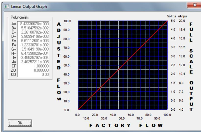
This screen shows the linear outputs and the corresponding flow rates. Adjustments made to the Full Scale, C-Factor, Zero Offset and Flow Cutoff will be reflected in this display.
