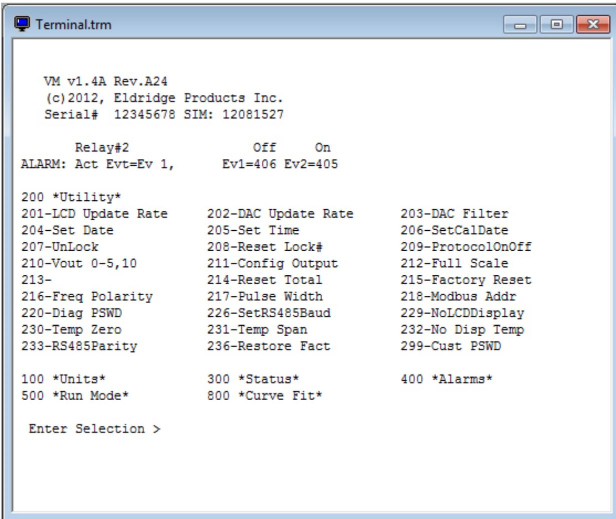
The 200 \*Utility\* Menu of the ValuMass™ Series 400 flowmeter includes a series of submenu items which allow you to easily change a wide variety of microprocessor parameters, such as the display update rate, the internal date and time, etc. Values for timing functions are in millisecond (ms) increments.
