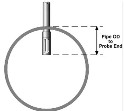
The calculation for the probe insertion depth (pipe OD to probe end) includes the point-of-average-flow, the slot in the protective sensor window, and the wall thickness of each nominal pipe size, as well as a further adjustment on smaller line sizes to be sure that the slot is fully inserted through the pipe wall. The C-Factor corrects the blockage effect created by inserting the probe assembly into the pipe to the depth listed.
