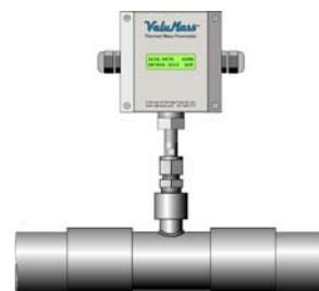
Inline flowmeters are calibrated with the sensing element mounted in place within the flow section. The sensor should not be removed as the accuracy of the flow signal will be slightly affected. Should it become necessary to remove the sensing element for any reason, the element should be replaced in the same alignment as it was originally positioned. Consult the factory before disassembling.
