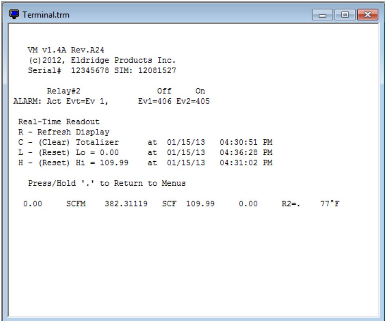
The **Real-Time Readout** commands are available while the flowmeter is in the basic Run Mode:
