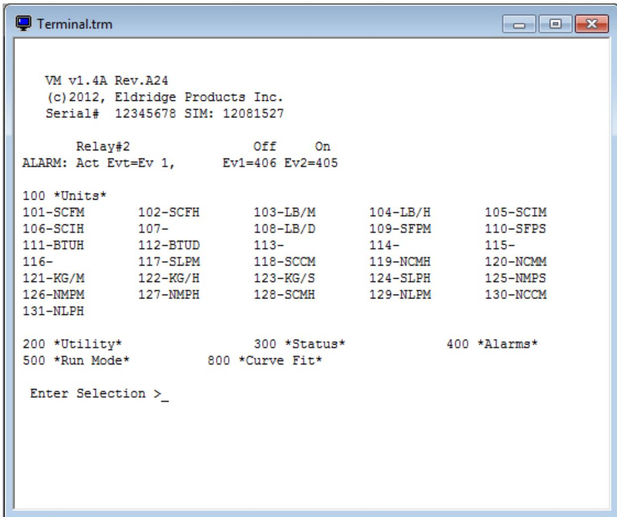
With the meter settings unlocked, type the menu number of desired engineering unit at the prompt and then press ENTER. The flowmeter will restart using new operational engineering units. The
