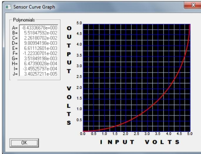
This screen shows the non-linear 0–5 VDC scaling of the bridge voltage and the Primary Coefficients used by the microprocessor to linearize the signal.
