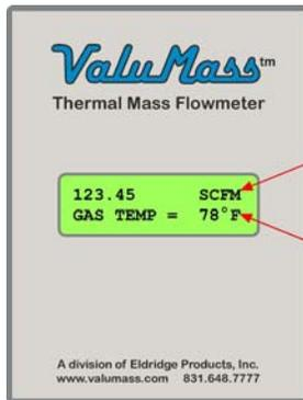
**Line 1 — Current Flow Rate** is the real-time flow rate in currently selected engineering units;
