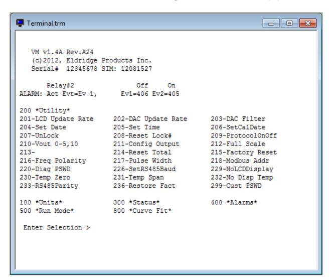
Although most settings are accessible by using the default user password of "9001", some of the parameters require a special password available only by contacting the factory. This has been instituted to prevent the accidental change of critical settings.
