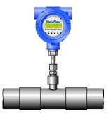
2" pipe. The standard end configuration is MNPT (male national pipe thread) threaded ends or Butt Ends for welding. If required, optional end mounting styles may be available (consult factory). Pipe sizes in excess of 2" require the insertion mounting style discussed below.
