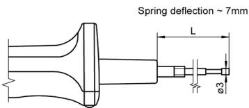
For surface measurement and immersion measurement
