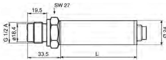
Type **FD8214M** membrane flush with front (welded with end of thread), internal thread G1/2" can be easily sterilized
