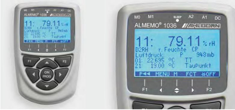
**Reference measuring instrument for humidity**
