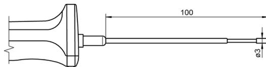
For surface measurement and immersion measurement
