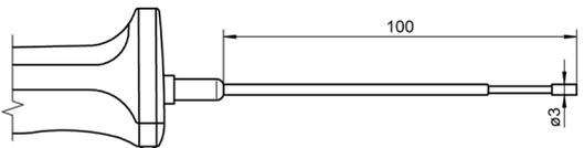
For surface measurement and immersion measurement
