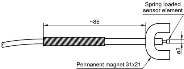
Magnet sensor For surface measurement
