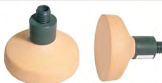
Sensor completely porous for measuring in thin layers of substrate.
