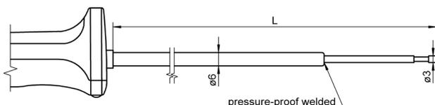
For surface measurement and immersion measurement
