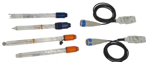
Transducer cable with various electrodes
