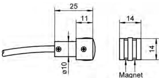
Magnet sensor for surface measurement
