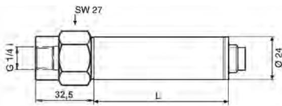
Type **FD 8214** standard version with internal thread G1/4"
