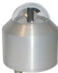
Probe for measuring global radiation FLA 613 GS-SDEK,
