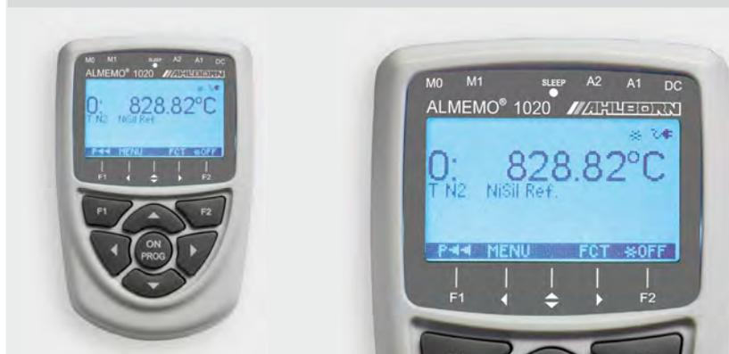
**Reference measuring instrument for temperature**
