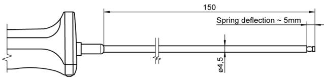
For surface measurement on level, metallic surfaces
