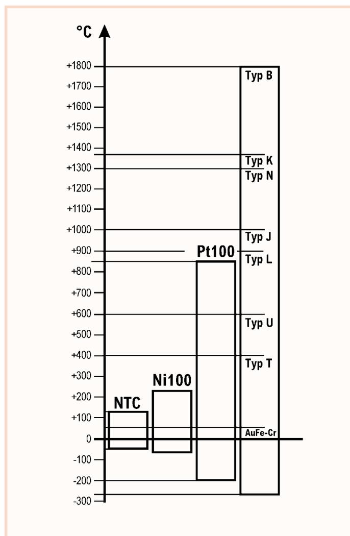
Selecting the right type of temperature sensor depends on your measuring task. For example, thermocouples, resistor-based sensors (Pt100 and Ntc) and pyrometers (infrared sensors) are available.
