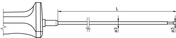
For surface measurement and immersion measurement
