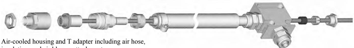
Air-cooled housing and T adapter including air hose, insulation, and air blower attachment
